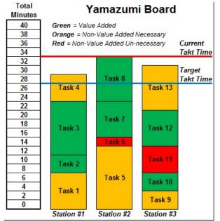
added (green), non-value added but necessary (orange) and non-value added and not necessary (red) tasks for assembly line workstation activities.
